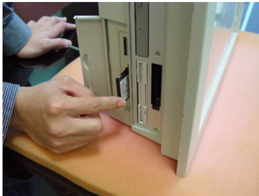
Figure 3.4: Inserting and ejecting a PCMCIA card
